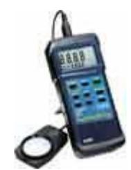
**Lux meter**: it is a device used for the measurement of illumination level. It consists of a photo cell which senses the light output, converts to electrical impulses which are calibrated as Lux.
